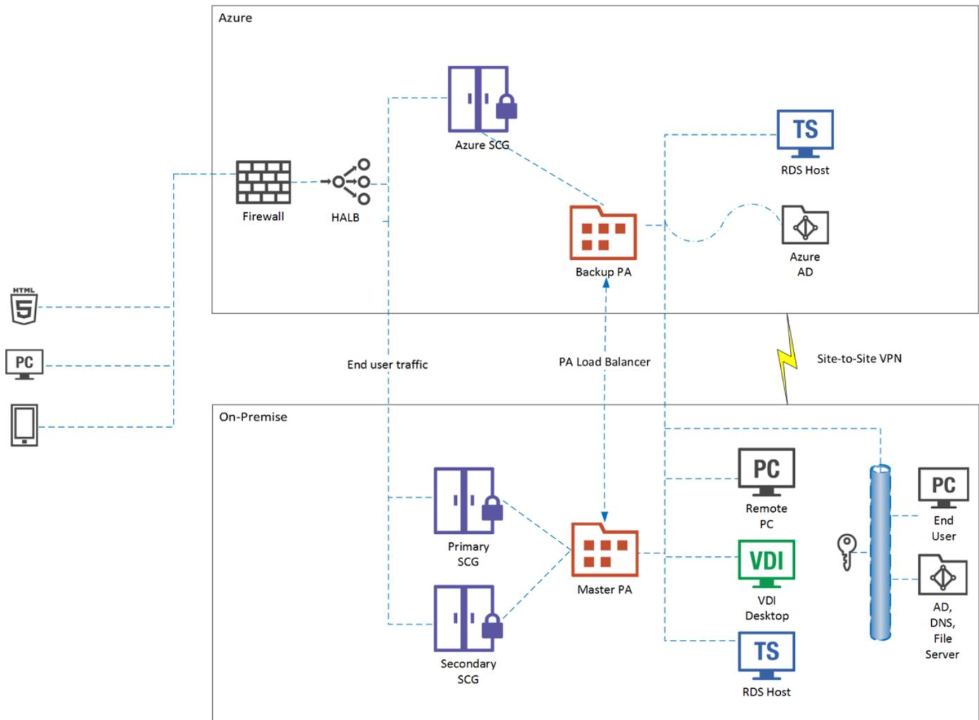
**Figure 5.** Typical Parallels Remote Application Server high availability deployment combining on premise HPE ProLiant DL380 Gen9 servers and Azure
