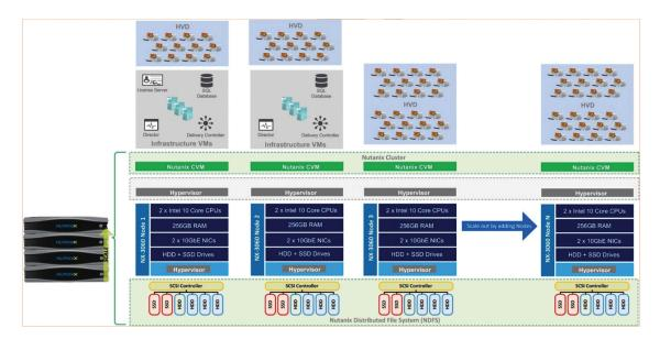
Figure 4. Logical View of the HVD Solution
