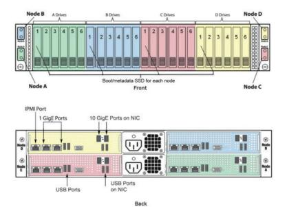
Figure 25. Nutanix NX-3000 Front and Rear View of Chassis depicting Nodes 1 to 4 (Nodes A to D)
