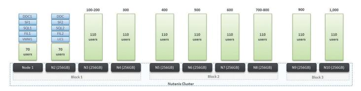
Figure 9. 1,000 HVD users - Virtual machine allocation in relation to Nutanix nodes
