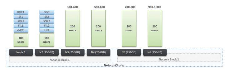
Figure 7. 1,000 RDSH Users - Virtual Machine allocation in relation to Nutanix Node
