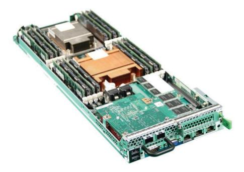
Figure 26. Nutanix NX-3000 Series Node - Physical View
