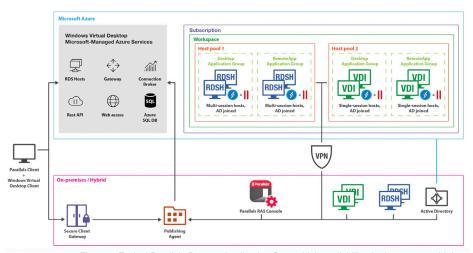
Figure 5. Typical Parallels Remote Application Server high availability deployment combining on-premises HPE ProLiant DL380 Gen10 servers and Azure
